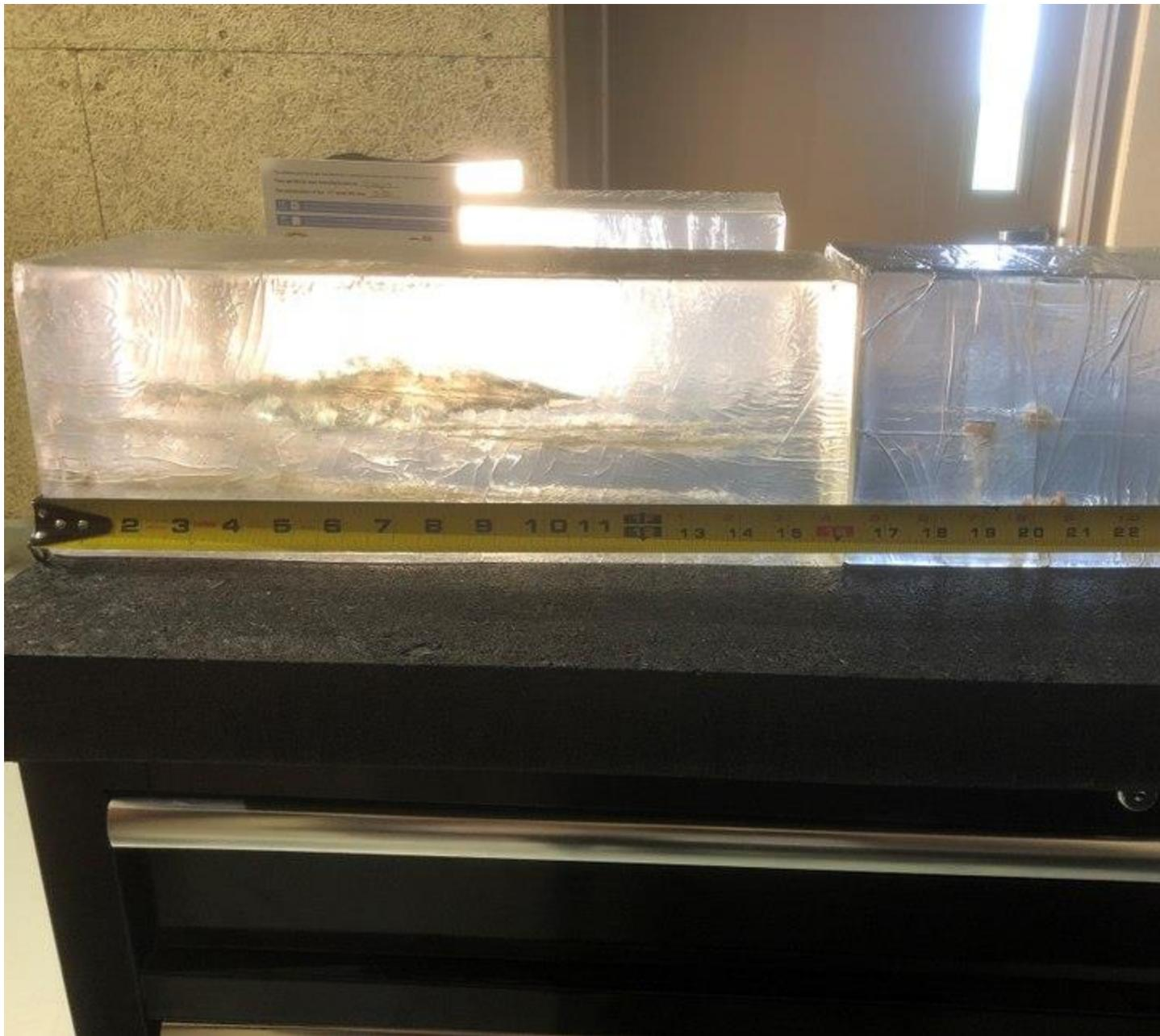
Bullets fired into the clear synthetic gelatin tended to expand less and penetrate more than they did in 10% organic gelatin. Shown is the 9mm Hornady Critical Duty 135+P. (Photo/Mike Wood)
