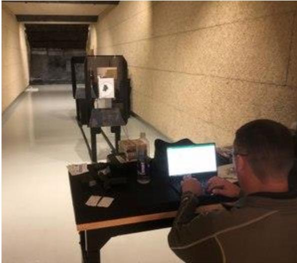
Meticulous records were kept during all phases of testing, documenting velocities, penetration depths, expansion and retained weight. (Photo/Mike Wood)
