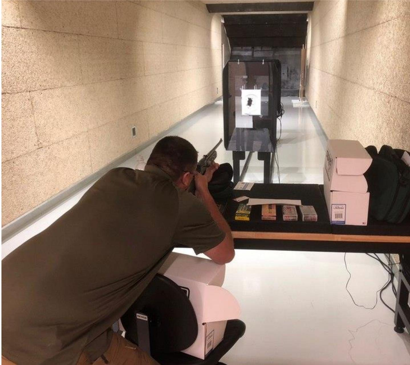
Chronographing the BB gun at the test facility, prior to firing calibration shots into the gel.
