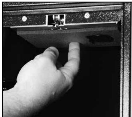
5. With the lid open, verify that the new code has been programmed and is functional by entering the new code. The safe motor should cycle after each correct entry.
