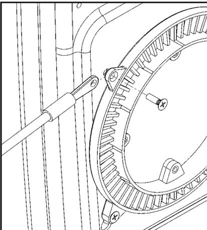
The Vehicle Safe attaches to the mounting plate using two clamping rings. The safe ships with one ring already attached to the back of the safe.
